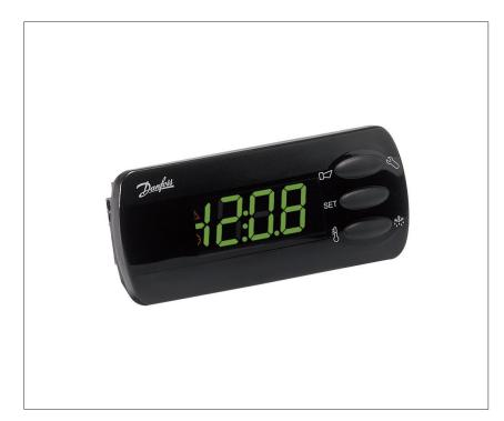
MMILDS is MCX's family remote interface. It's fitted with a LED display for displaying data from a MCX or from 2 probes that can be locally connected. The connection with any MCX controller is through the CAN bus network. The power supply can come from controller which it is connected.
